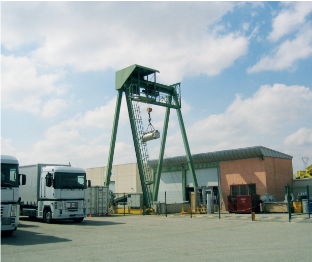
Drop test of a packaging intended for the transport of spent fuel
