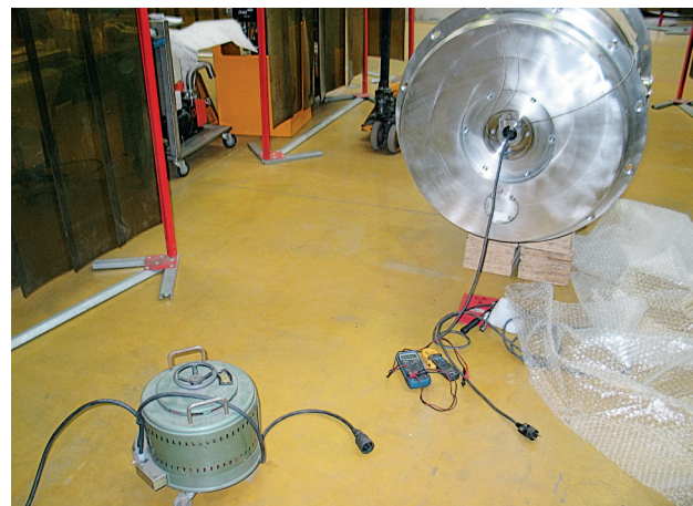
Thermal test on a transport packaging
